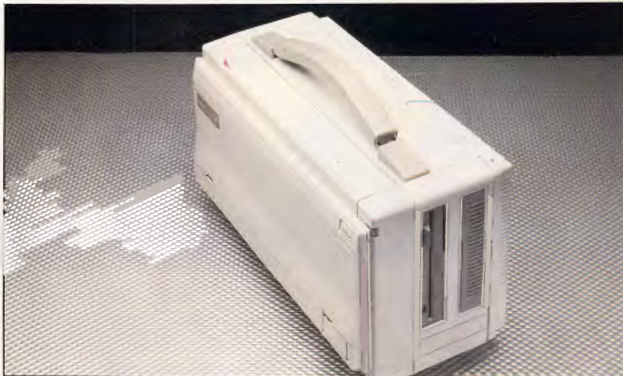
Compaq maintains that 5 \frac{1}{4} in floppy drives are the industry standard and so has not been tempted by 3.5in ones. The 1.2Mbyte drive can be replaced with a 360k unit
