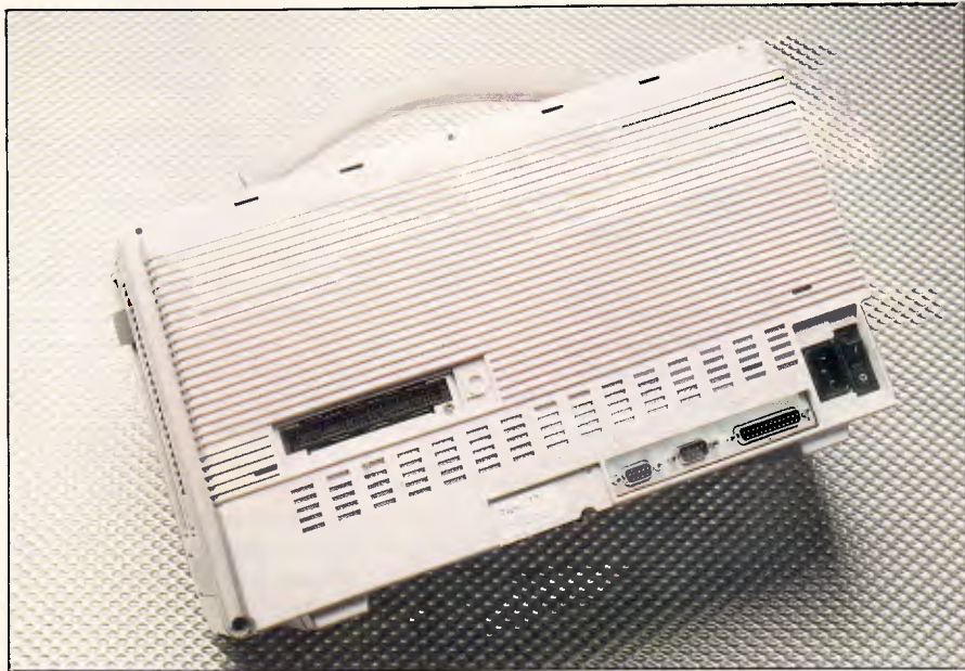
The centrally-mounted expansion slot takes snap-on boxes: one of which holds a 40Mbyte tape streamer: the other takes expansion cards
